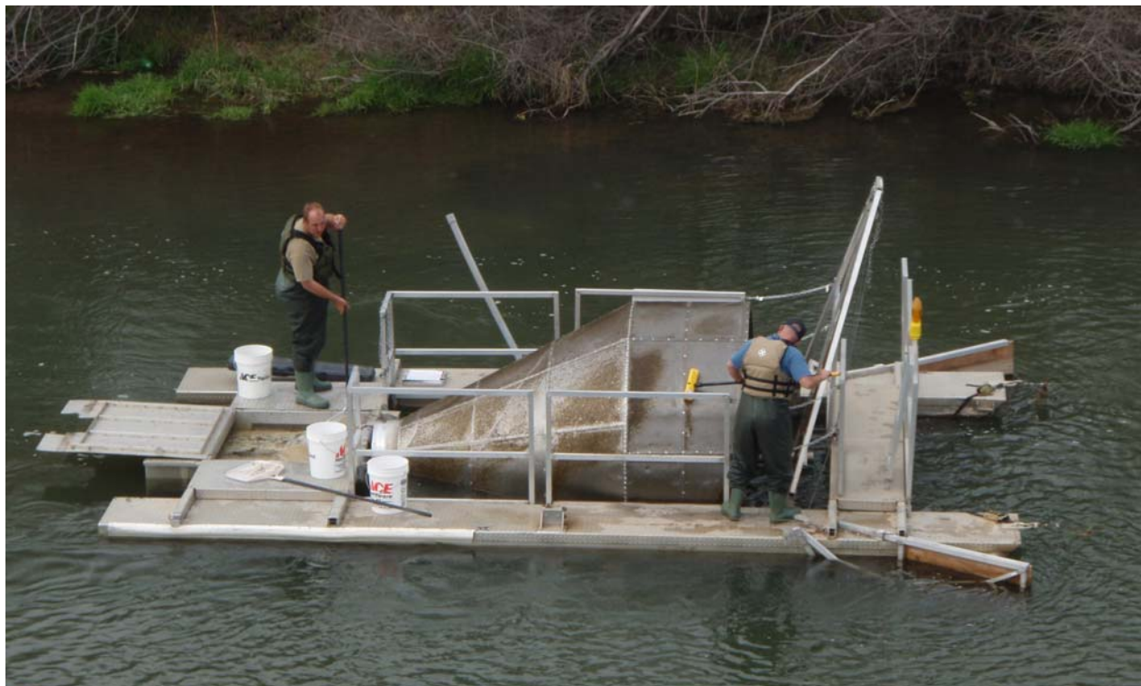
Figure 2. Waterford rotary screw trap with “wings” attached to the upstream end of the pontoons.
